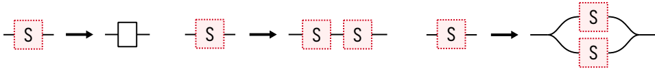
Figure 5.5: A context-free monoidal grammar of series-parallel graphs, with start symbol S , over the alphabet containing a “node”, “branch”, and “merge” generators.
