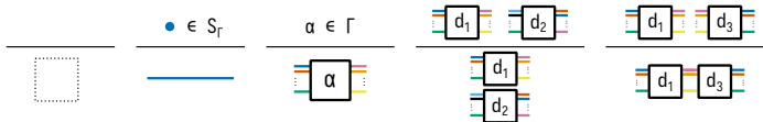
Fig. 2: The free strict monoidal category over a polygraph \Gamma has set of objects S_\Gamma^* and morphisms string diagrams given inductively over the generators of \Gamma as above quotiented by the equivalence relation generated by planar isotopy of diagrams, keeping left and right boundaries fixed. The leftmost rule denotes the empty diagram. We use colours to indicate sorts.
